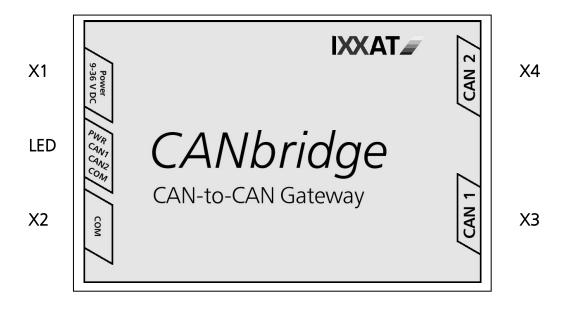
Fig. 2-1: Pin allocation aluminum version
